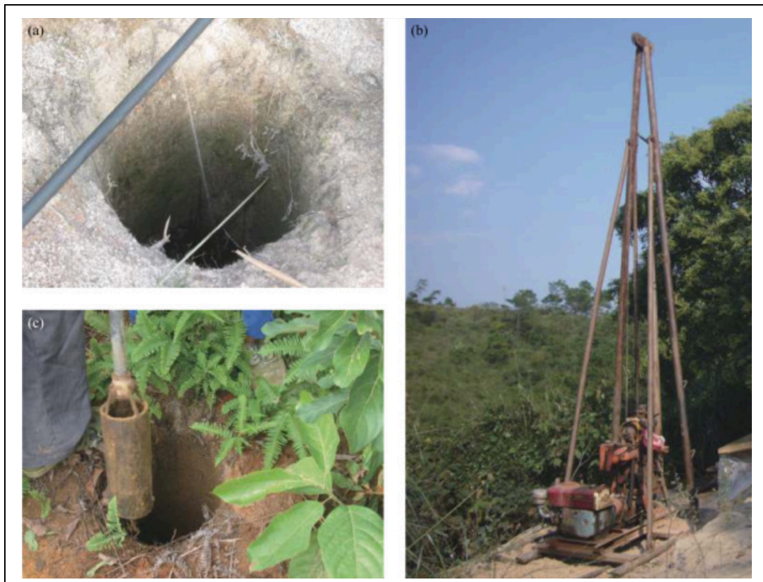
Figure 2: Simple Drilling Equipment and Machinery for the Ion Adsorption REE Exploration
