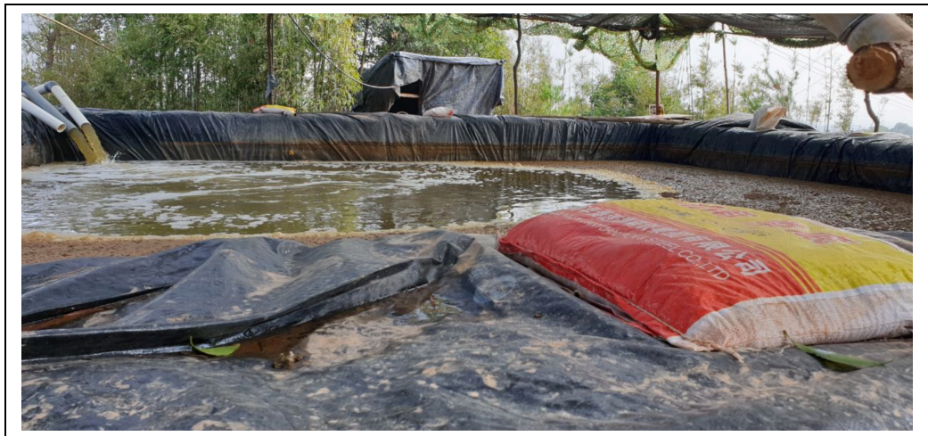
Plate 5: Storage of Leaching Solution Located at High Elevation Tank as Part of the Reticulation Network System for the In-Situ Leaching Mining Operation of Ion-Adsorption Clay Deposit in Guangxi Rare Earth, China
