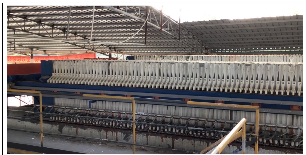
Plate 10: Filter Press for Water Separation of the Precipitated RE Carbonate
