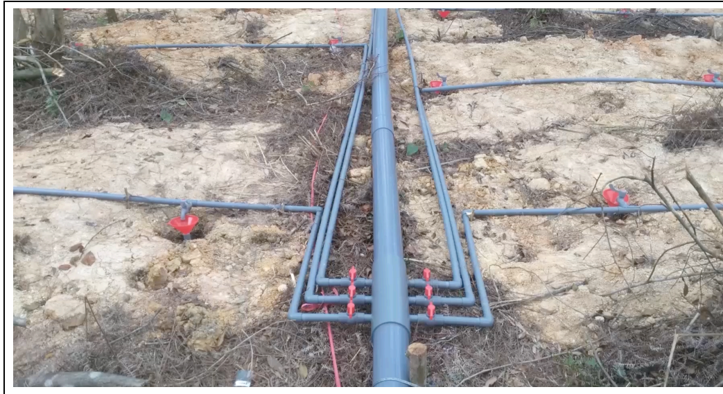
Plate 4: Another View of Leaching Solution Reticulation Network System for the In-Situ Leaching Mining Operation of Ion-Adsorption Clay Deposit in Guangxi Rare Earth, China
