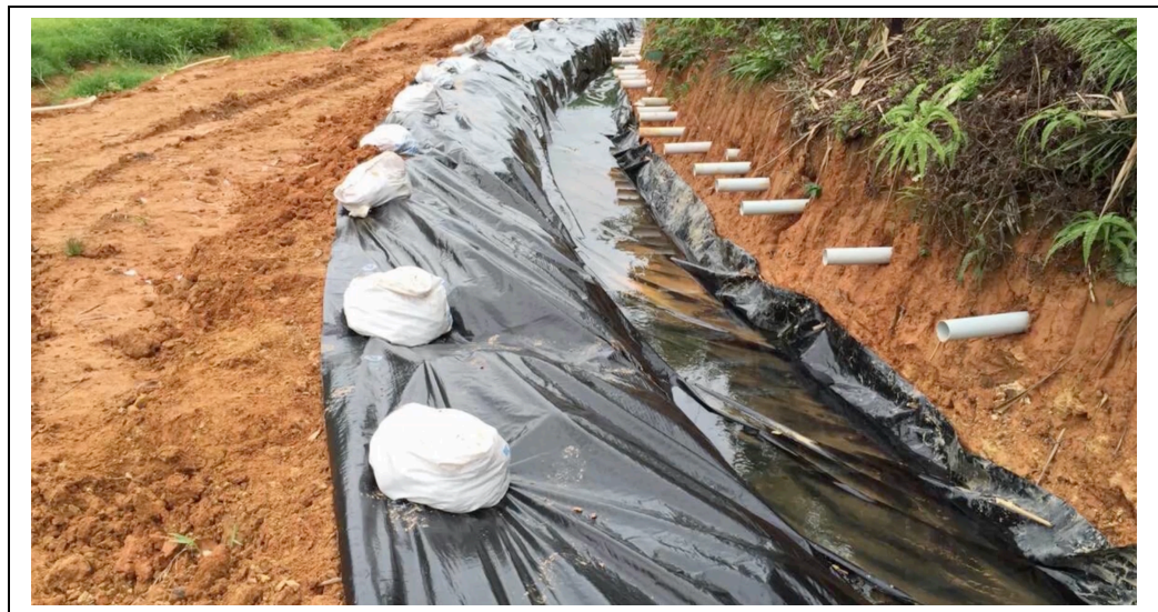
Plate 7: Another View of Diversion Holes of Pregnant Solution and the Collection Ditch as Part of the Reticulation Network System for the In-Situ Leaching Mining Operation of Ion-Adsorption Clay Deposit in Guangxi Rare Earth, China
