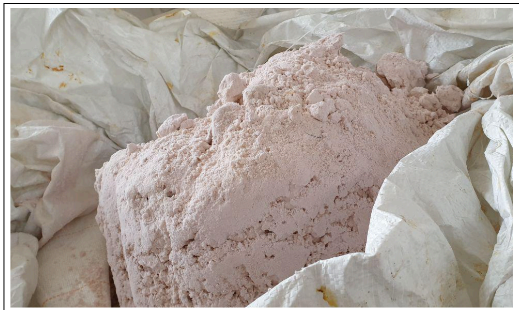
Plate 1: Intermediate REE Product – RE Carbonate, Final Mine Product for Further Processing into REE Oxide and Crack into 16 REE at Guangxi Rare Earth, a Unit of Chinalco Rare Earth & Metals Co. Ltd.
