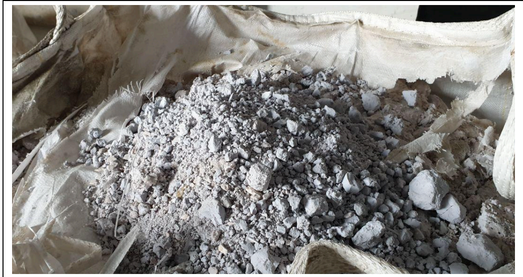
Plate 3: Intermediate REE Product – RE Oxide for Further Processing to Crack into 16 Elements of RE, Final Product of Ion-Adsorption RE Clay Deposit, Produced at Guangxi Rare Earth, a Unit of Chinalco Rare Earth & Metals Co. Ltd.
