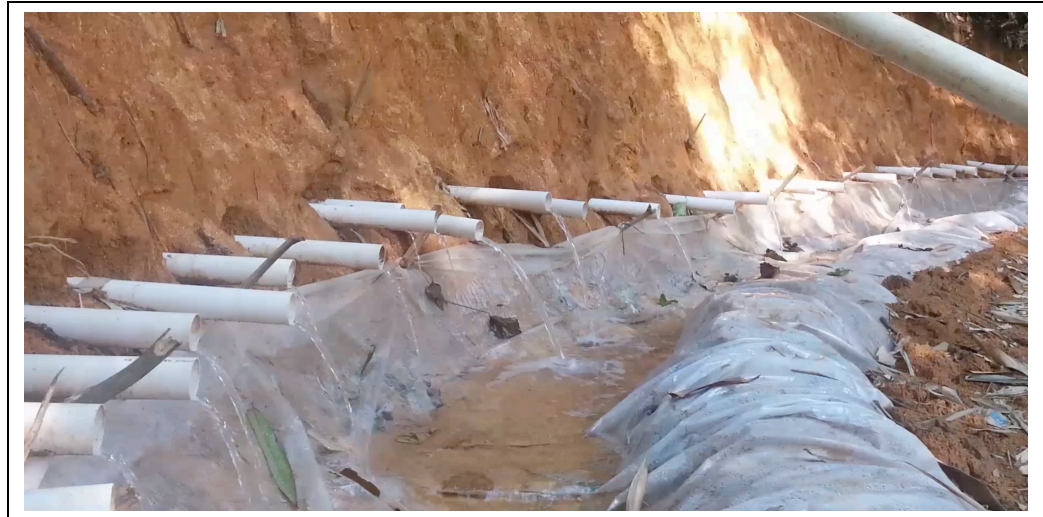
Plate 6: Diversion Holes of Pregnant Solution and the Collection Ditch for the In-Situ Leaching Mining Operation of Ion-Adsorption Clay Deposit in Guangxi Rare Earth, China
