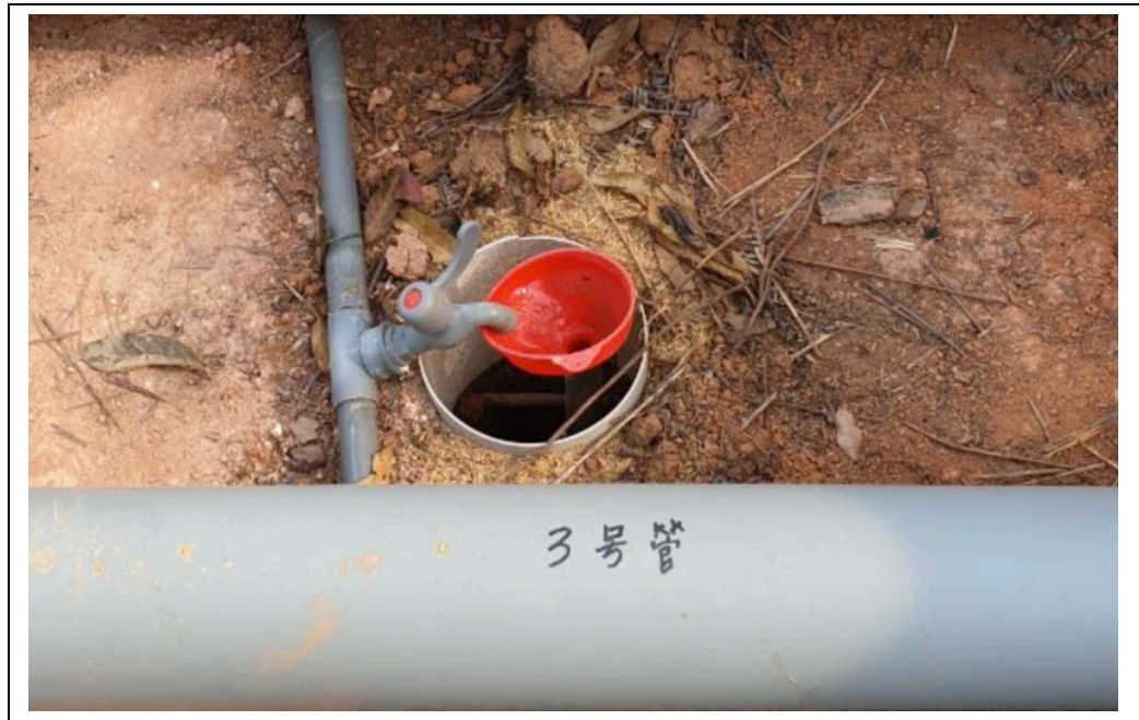
Plate 2: Dripping of Leaching Solution to the Ion-Adsorption RE Clay Deposit through the Injection Hole at the In-Situ Leaching Mining Operation in Guangxi Rare Earth, China
