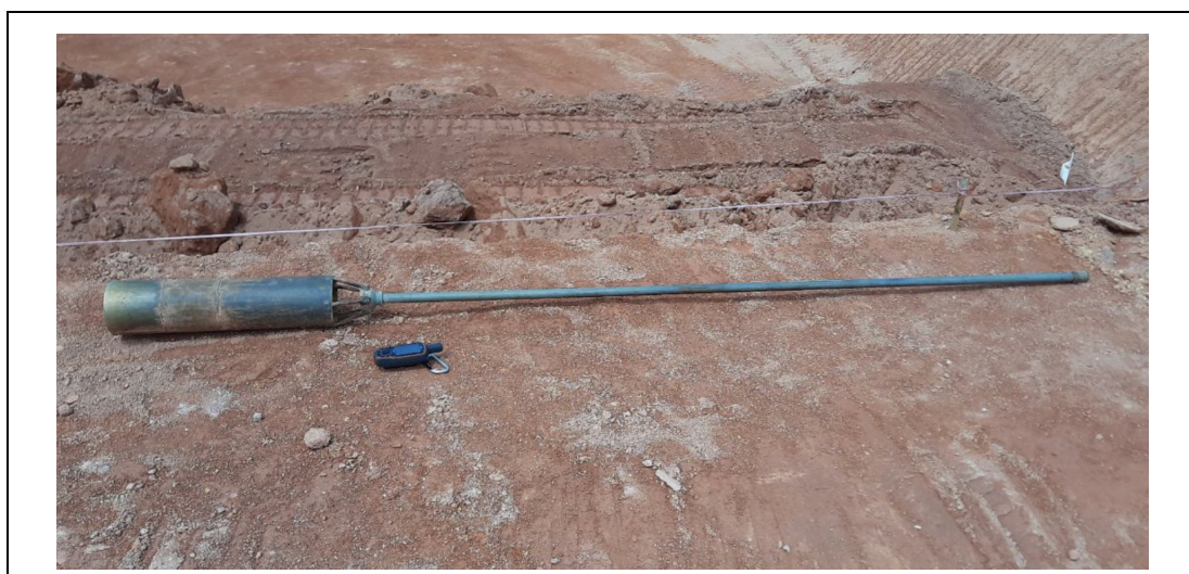
Figure 3: Gannan Drill, Simple Drilling Equipment for the Ion Adsorption REE Exploration
