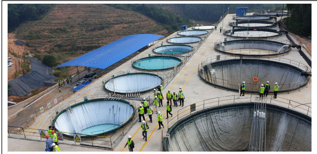
Plate 8: Processing Pools as Part of RE Carbonate Processing Facility at an In-Situ Leaching Mining Operation of Ion-Adsorption Clay Deposit in Guangxi Rare Earth, China
