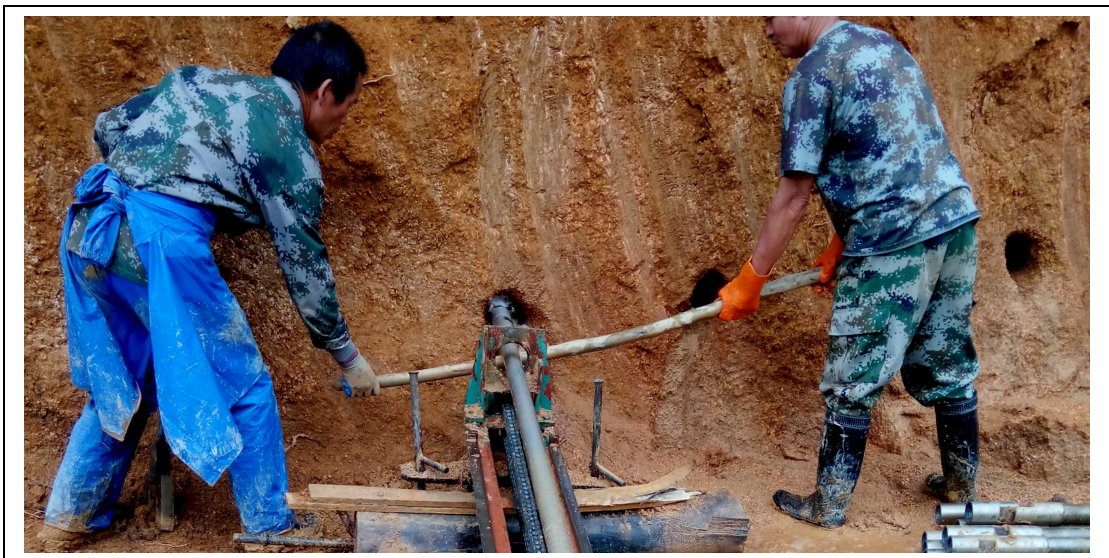
Plate 2: Preparation of Pregnant Solution Diversion Holes for the In-Situ Leaching Mining Operation of Ion-Adsorption Clay Deposit in Guangxi Rare Earth, China
