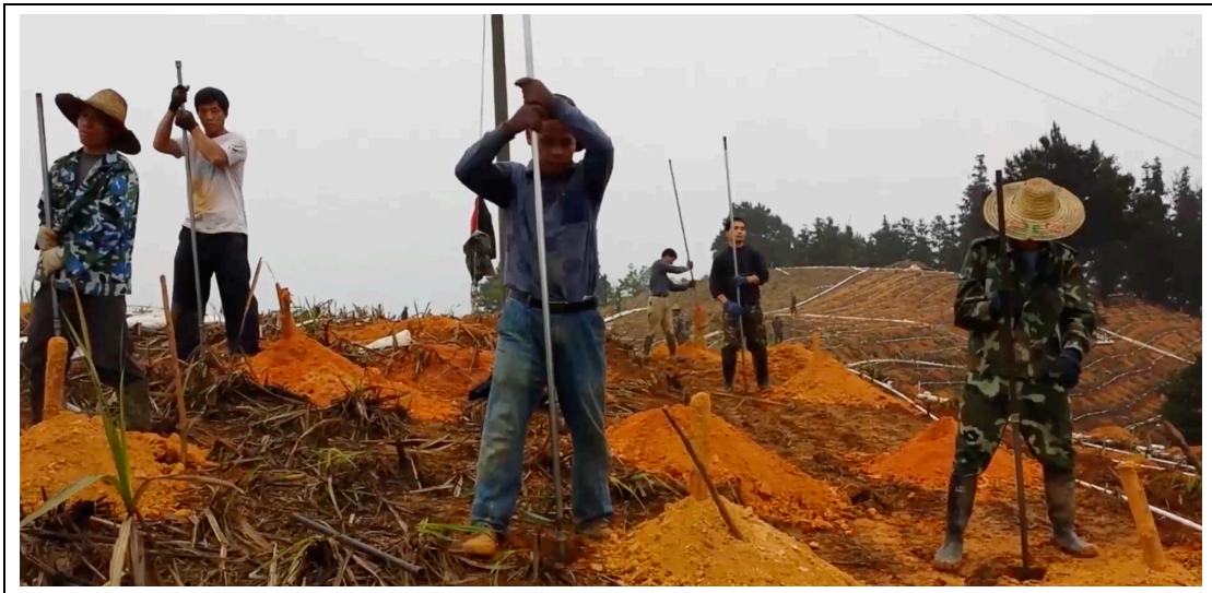
Plate 1: On-site Manual Preparation of Liquid Injection Holes for the In-Situ Leaching Mining Operation of Ion-Adsorption Clay Deposit in Guangxi Rare Earth, China
