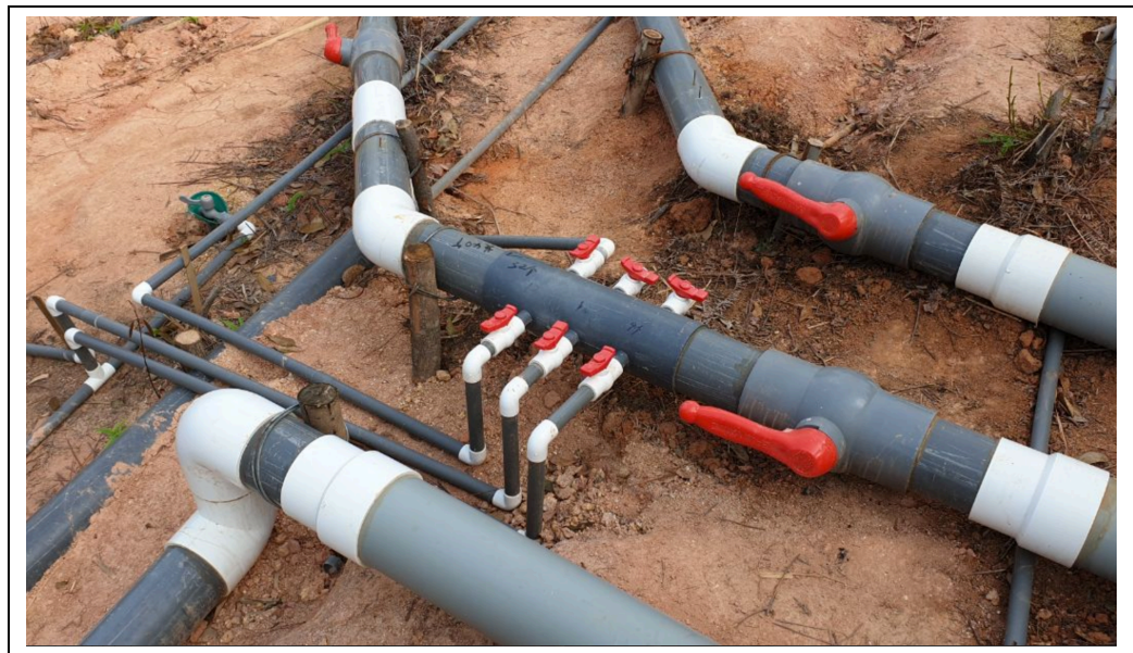
Plate 3: Leaching Solution Reticulation Network System for the In-Situ Leaching Mining Operation of Ion-Adsorption Clay Deposit in Guangxi Rare Earth, China
