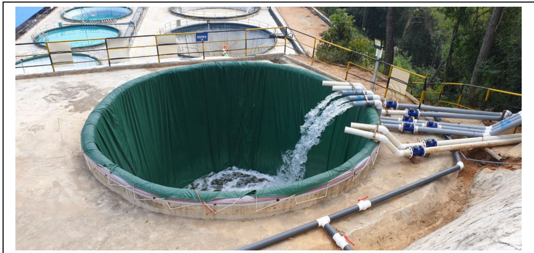
Plate 9: Processing Pools as Part of RE Carbonate Processing Facility at an In-Situ Leaching Mining Operation of Ion-Adsorption Clay Deposit in Guangxi Rare Earth, China
