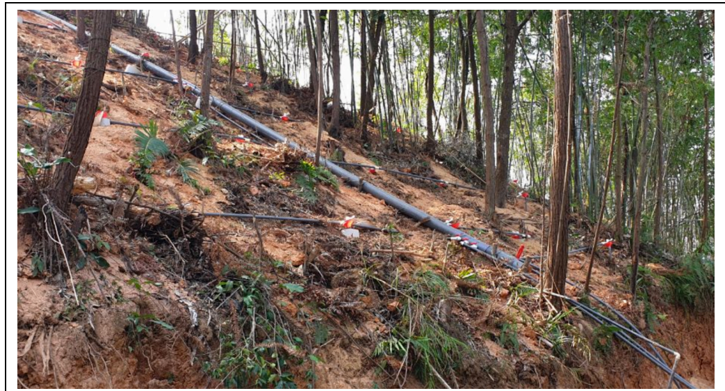
Plate 1: Piping Network System for the In-Situ Leaching Mining Operation of Ion-Adsorption Clay Deposit in Guangxi Rare Earth, China
