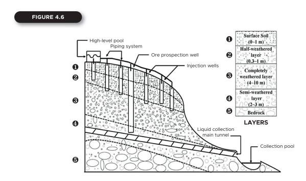
Figure 4.6: Schematic diagram of in-situ leaching mining set-up (Vahidi, Navarro & Zhao, 2016)
