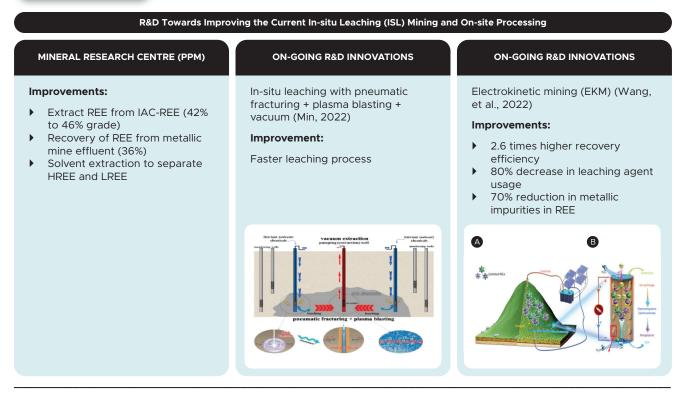
Figure 4.7: R&D initiatives to improve the current ISL mining and on-site processing methods
